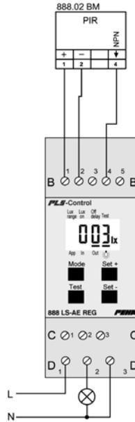
**Function 6: Automatic ON and OFF triggered by motion detector. Light sensor not in use**
