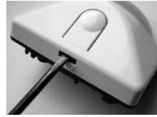
The motion detector has two possible settings. The designer cover on the top must be opened to use the adjusting potentiometer.
